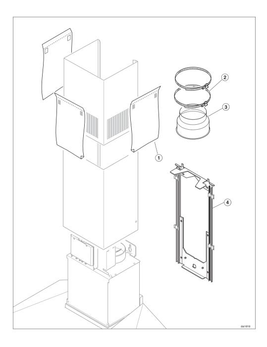
① **3 protective shields** to prevent scratches to the chimney during installation.
